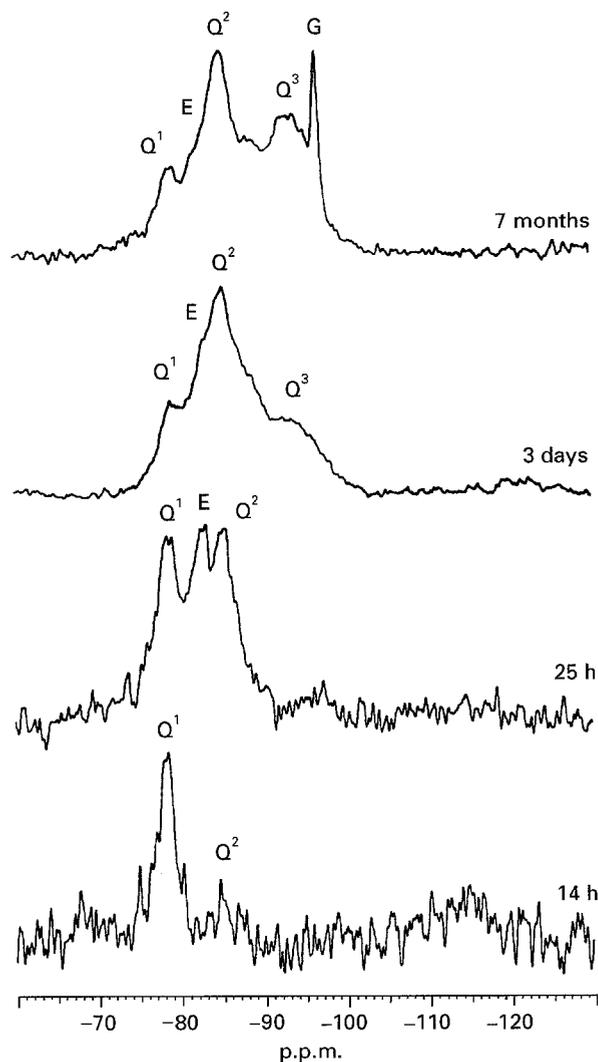
Figure 8 Selected  $^{29}\text{Si}$  CPMAS NMR spectra showing the reaction of 5M KOH solution with a blend of tricalcium silicate and silica. 10 Hz of exponential linebroadening was applied to these spectra. The nature of the peaks E and G is discussed in the text.
