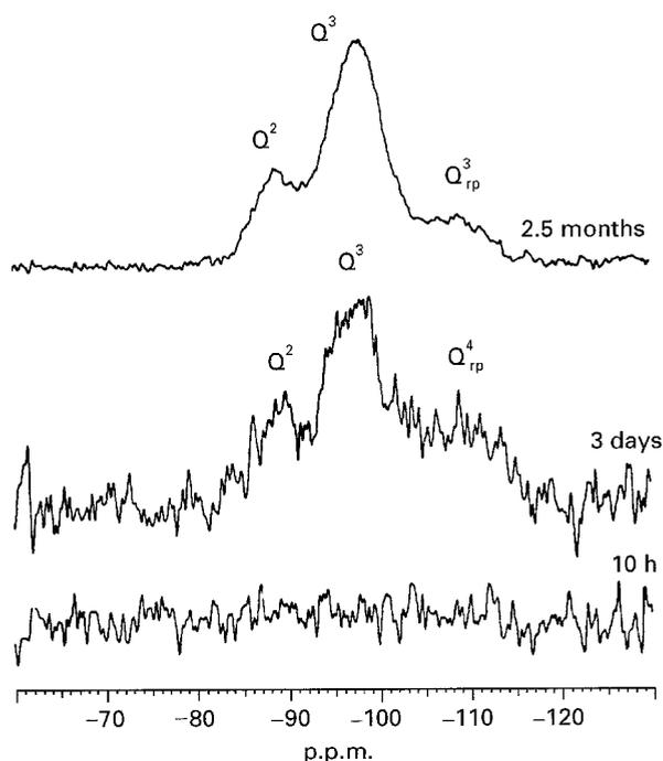
Figure 4 Selected  $^{29}\text{Si}$  CPMAS NMR spectra showing the reaction of 5 M KOH solution with silica. 10 Hz of exponential linebroadening was applied to these spectra.  $Q_{rp}^4$  denotes  $Q^4$  species contained in the reaction products.
