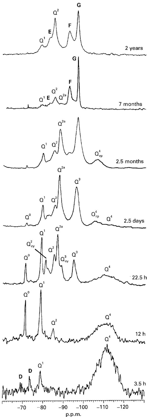
Figure 7 Selected  $^{29}\text{Si}$  MAS NMR spectra showing the reaction of 5M KOH solution with a blend of tri-calcium silicate and silica. 10Hz of exponential linebroadening was applied to these spectra. Notation as Fig. 3. The nature of the peaks D, E, F, G and  $Q^{2a}$  is discussed in the text.
