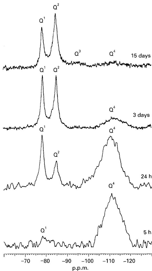
Figure 1 Selected  $^{29}\text{Si}$  MAS NMR spectra showing the reaction of calcium oxide with water and silica. 5 Hz of exponential line-broadening was applied to these spectra, except at early ages, when 20 Hz was applied. The  $Q^n$  notation is described in the text. Hydration times are indicated on the figures.
