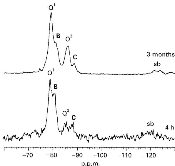
Figure 6 Selected  $^{29}Si$  CPMAS NMR spectra showing the reaction of 5 M KOH solution with tricalcium silicate. 5 Hz of exponential linebroadening was applied to these spectra. Notation as Fig. 5.
