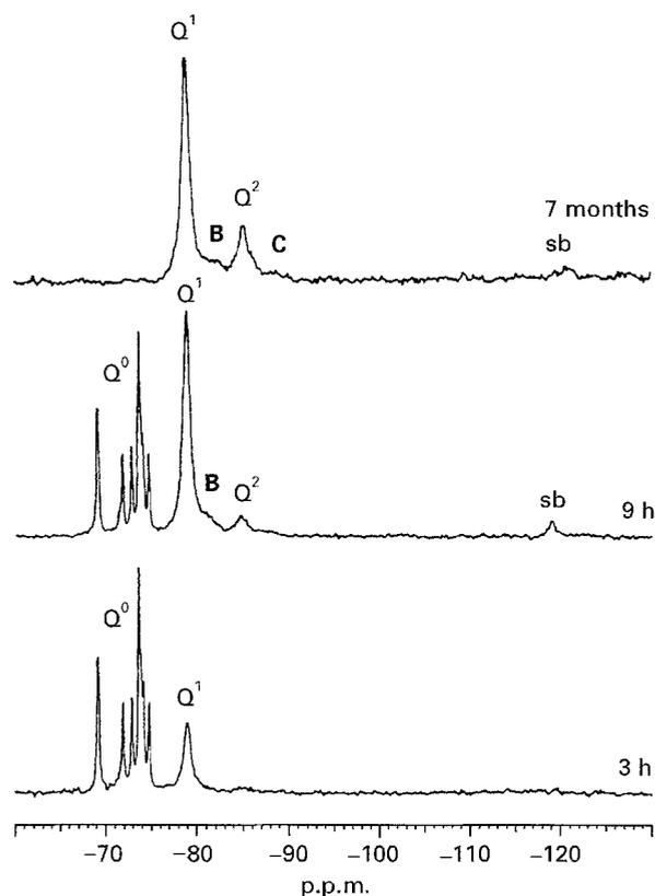
Figure 5 Selected  $^{29}Si$  MAS NMR spectra showing the reaction of 5 M KOH solution with tricalcium silicate. 5 Hz of exponential linebroadening was applied to these spectra. The nature of the peaks **B** and **C** is discussed in the text. Spinning sidebands are indicated by **sb**; they are an artifact of the MAS technique.
