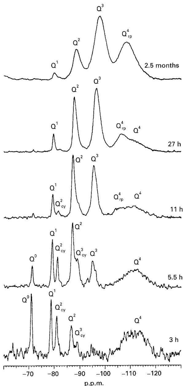
Figure 3 Selected  $^{29}\text{Si}$  MAS NMR spectra showing the reaction of 5 M KOH solution with silica. 10 Hz of exponential linebroadening was applied to these spectra. The notation  $Q_{cy}^2$  and  $Q_{cy}^3$  denotes  $Q^2$  and  $Q^3$  species contained in cyclic trimers;  $Q_{rp}^4$  denotes  $Q^4$  species contained in the reaction products.
