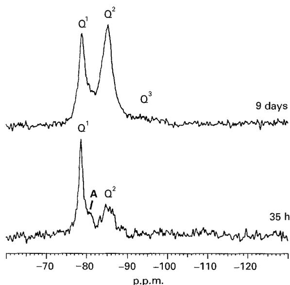
Figure 2 Selected  $^{29}\text{Si}$  CPMAS NMR spectra showing the reaction of calcium oxide with water and silica. 5 Hz of exponential line-broadening was applied to these spectra. The nature of the peak A is described in the text.
